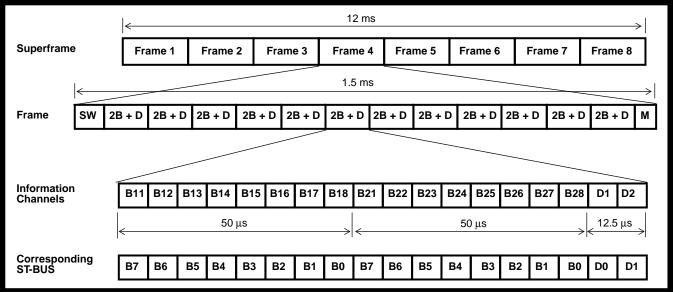
Figure 4 - Frame Structure
