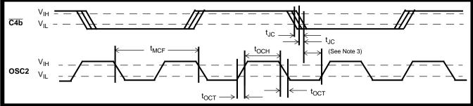
Figure 15 - External Clock Timing in LT Mode
