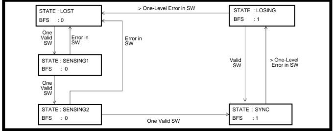
Figure 5 - Frame Synchronization State Diagram
