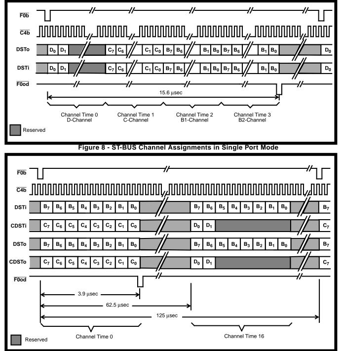
Figure 9 - ST-BUS Channel Assignment in Dual Port Mode
