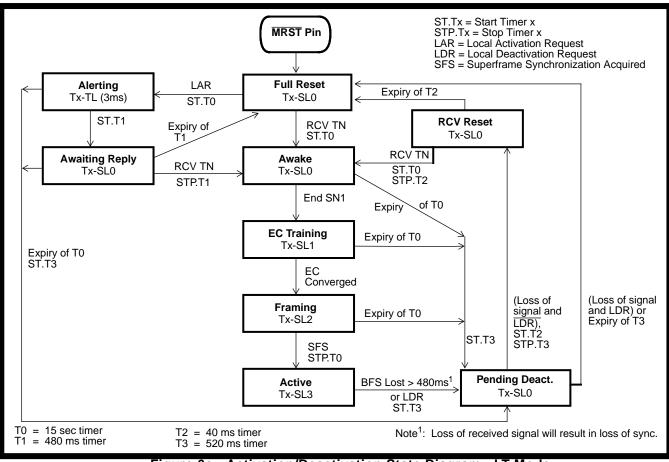
Figure 6a - Activation/Deactivation State Diagram - LT Mode
