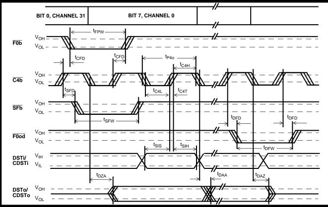
Figure 17 - ST-BUS Timing NT Mode
