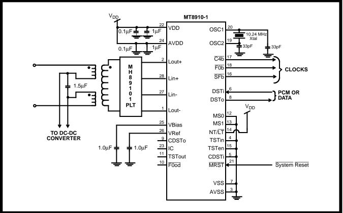
Figure 12 - Typical Connections for NT Mode (Single Port)
