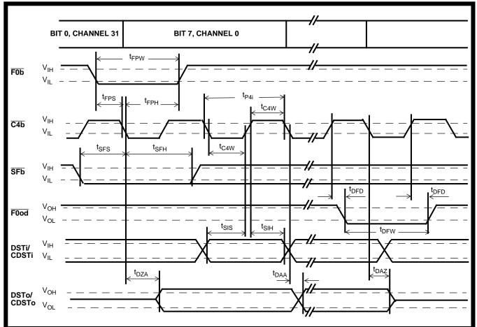
Figure 16 - ST-BUS Timing LT Mode
