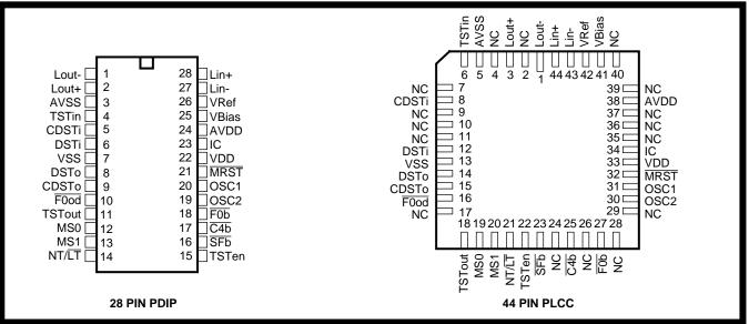
Figure 2 - Pin Connections
