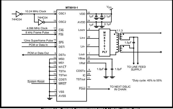
Figure 11 - Typical Connections for LT Mode (Single Port)
